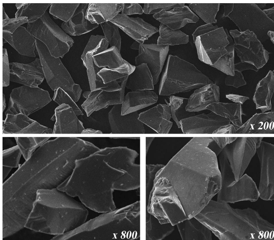
**Figure 4.** SEM pics of the SiC-100 surface shape.
