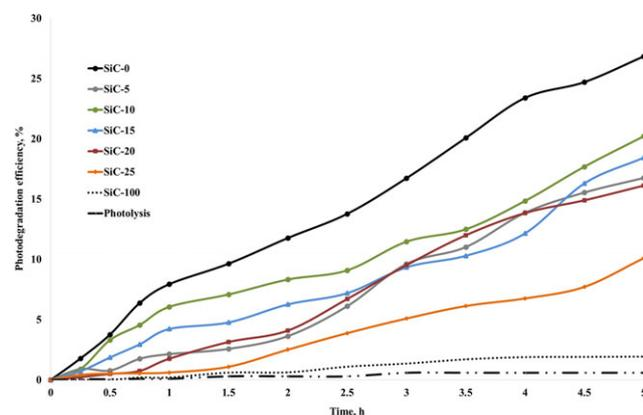
**Figure 9.** Photocatalytic efficiency of  $\text{TiO}_2/\beta\text{-SiC}$  catalysts composition in methyl orange (MO) degradation under 100 W UV lamp radiation.
