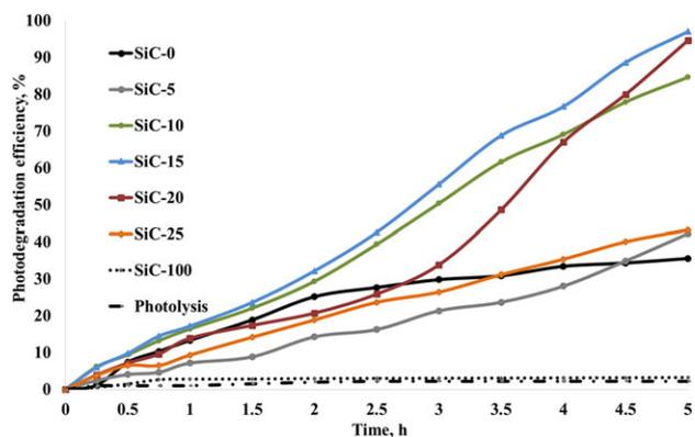
**Figure 8.** Photocatalytic efficiency of  $\text{TiO}_2/\beta\text{-SiC}$  catalysts composition in methylene blue (MB) degradation under 100 W UV lamp radiation.
