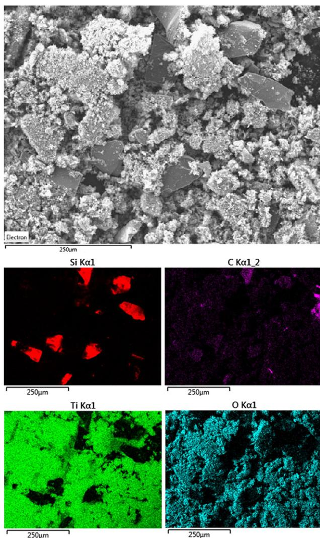
Figure 5. EDS elements mapping the surface of the SiC-15 catalyst.
