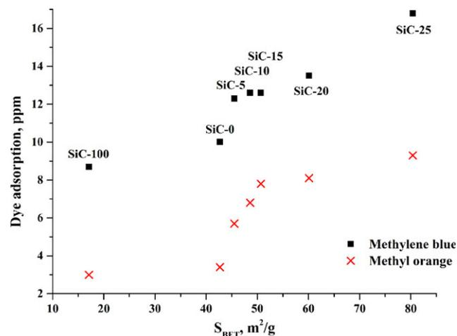
**Figure 7.** The correlation between BET catalysts surface area and the MB and MO adsorption level after 1 h of 100 ppm solution mixing with the catalyst concentration of 0.5 g L<sup>-1</sup>. [Color figure can be viewed at [wileyonlinelibrary.com](http://wileyonlinelibrary.com)]
