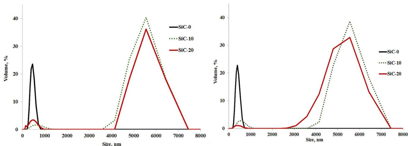
**Figure 6.** Catalysts particle size distribution measured with DLS method after the time of 5 min (A) and 15 min (B) sonication.
