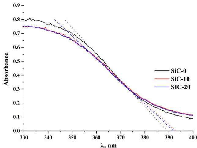
**Figure 3.** UV-Vis-DR results for the graphical Eg determination.
