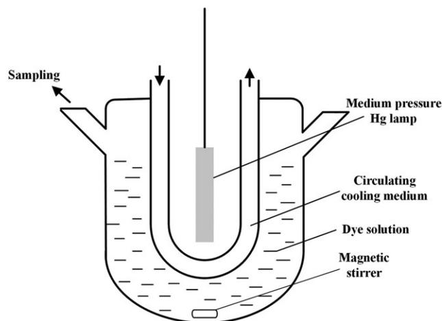
**Figure 1.** Experimental setup for photocatalytic degradation.
