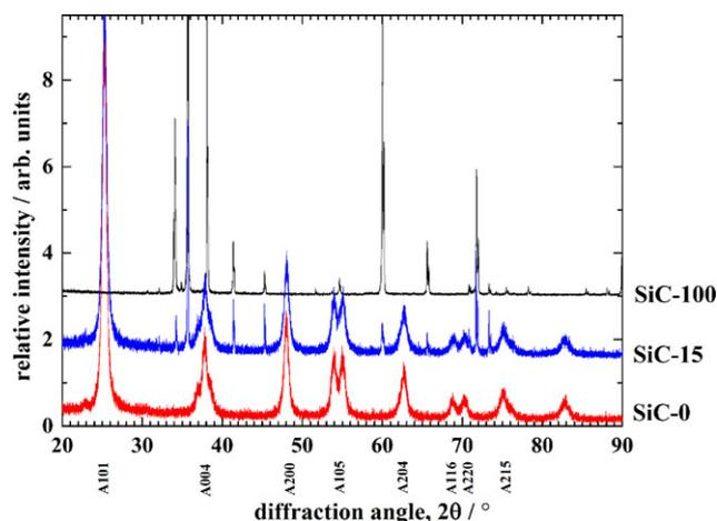
**Figure 2.** Raw powder diffraction patterns (with  $K\alpha_2$  intensities included) recorded for SiC-0, SiC-15 and SiC-100. The patterns are shifted along the intensity scale for clarity. Assignment of Miller indices was based on literature (26,27).
